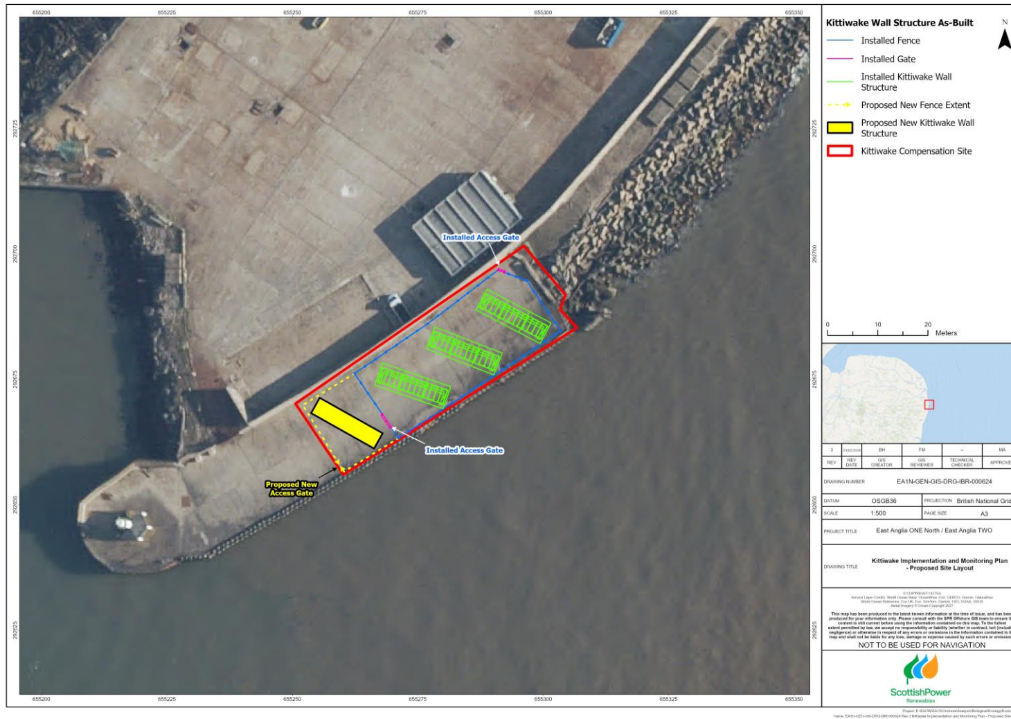
Figure 5: Proposed site layout of kittiwake wall structures at the port of Lowestoft
